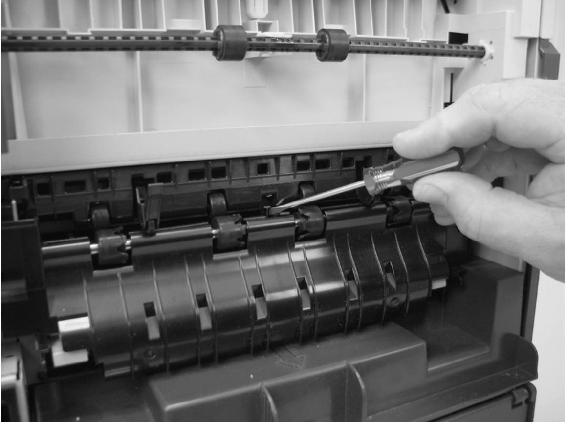
Figure 7-5 Checking the fuser delivery sensor
