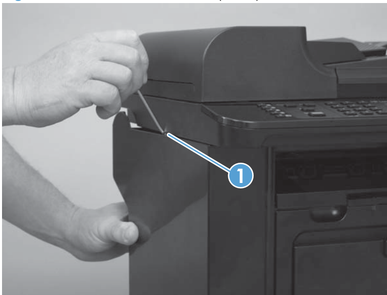
Figure 1-15 Remove the left cover (4 of 5)
