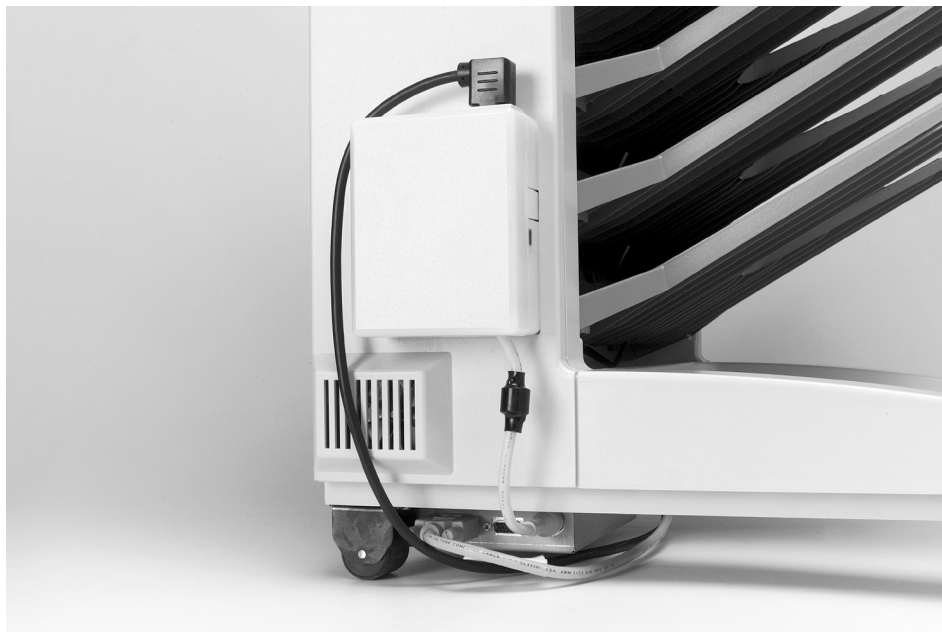
Figure 7-24 8-bin Mailbox Power Supply Test Mode Switch
