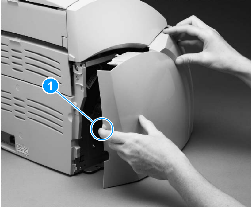
Figure 24. Removing the left side cover
