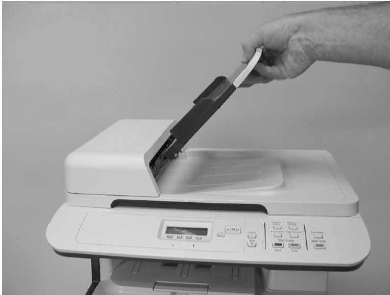
Figure 6-24 Remove the ADF input tray
