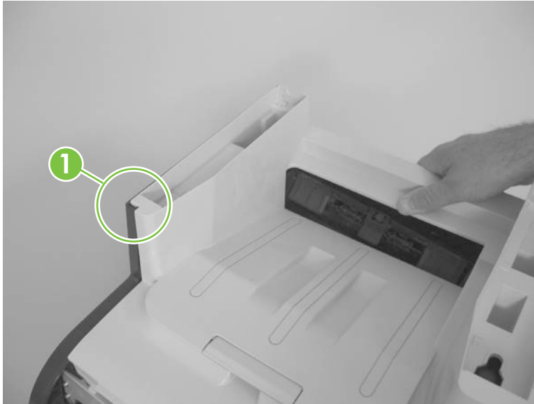
Figure 6-97 Reinstall the upper-cover assembly (1 of 3)
