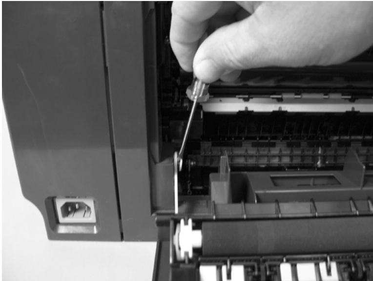
Figure 6-44 Remove the Rear-door stopper and link cap (simplex product) (2 of 2)
