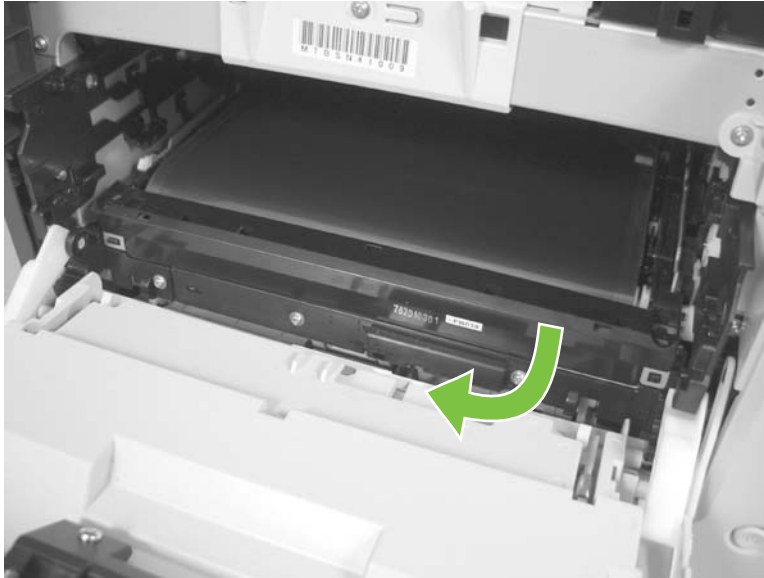
Figure 6-30 Remove the ITB (2 of 6)
