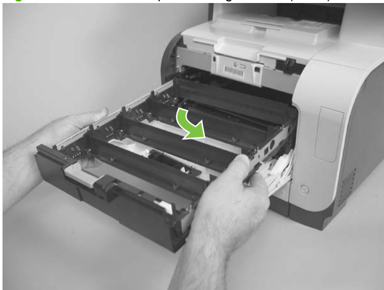
Figure 6-27 Remove the print-cartridge drawer (2 of 3)
