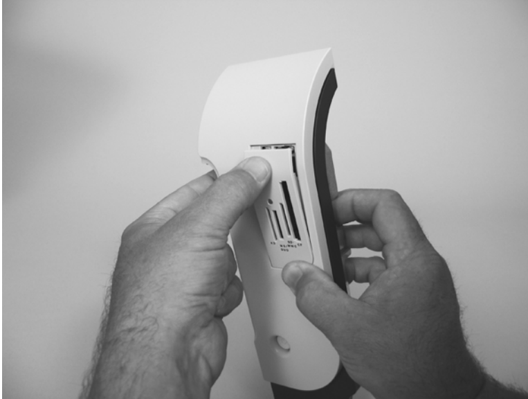
Figure 6-133 Reinstall the memory-card cover and PCA (2 of 2)
