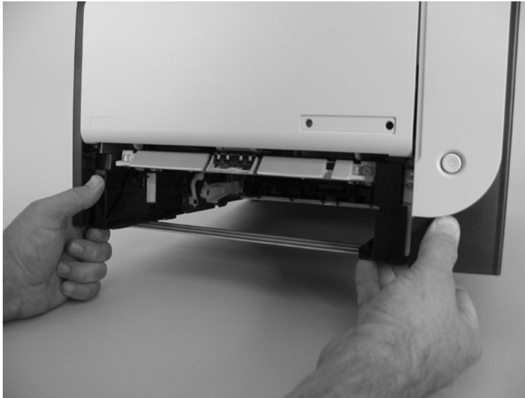
Figure 6-9 Remove the pickup roller (1 of 2)
