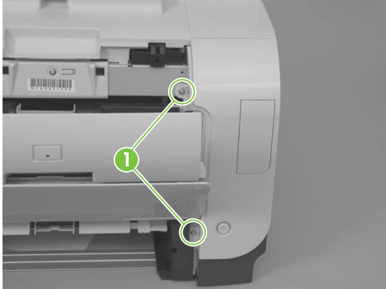
Figure 6-120 Remove the right-front cover and power button (1 of 5)
