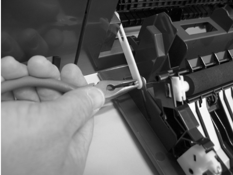
Figure 6-45 Remove the rear door (simplex product) (1 of 4)
