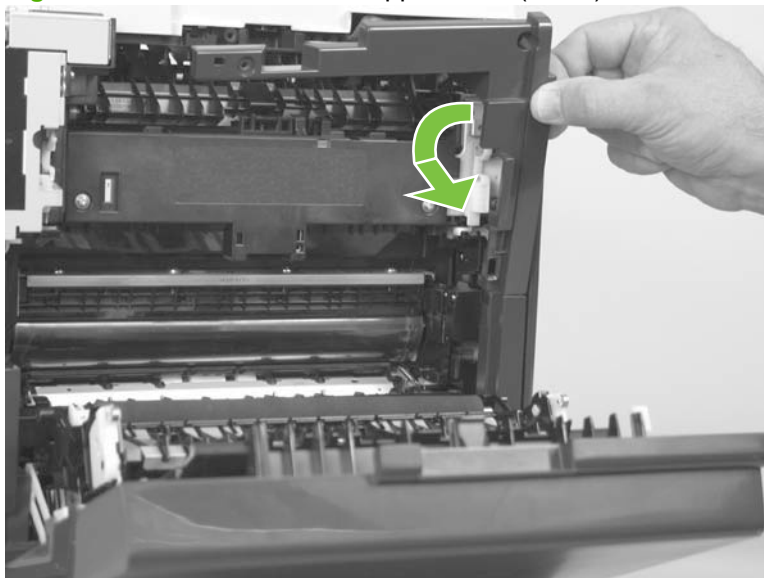
Figure 6-67 Remove the rear-upper cover (2 of 2)
