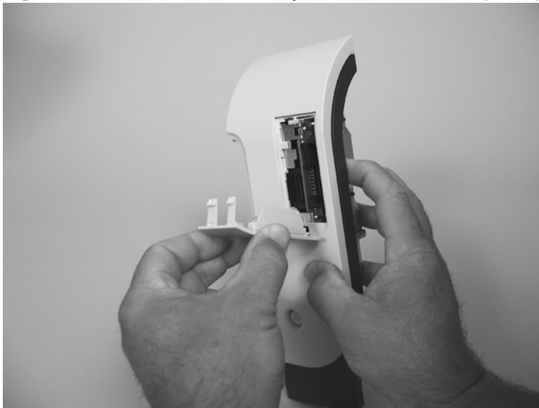
Figure 6-132 Reinstall the memory-card cover and PCA (1 of 2)
