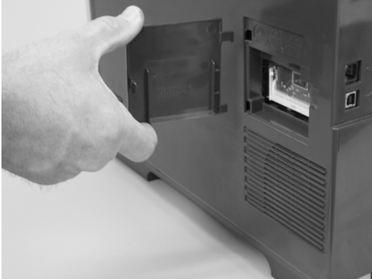
Figure 6-25 Remove the DIMM cover
