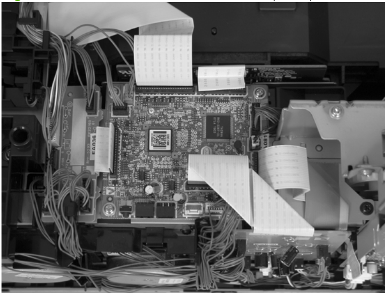
Figure 6-60 Remove the DC controller PCA (1 of 2)
