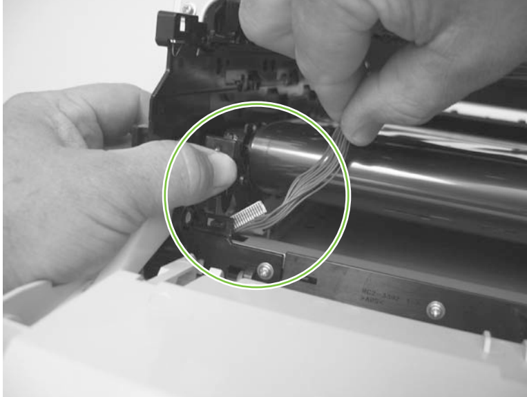
Figure 6-116 Reinstall the color-misregistration sensor assembly PCA (1 of 2)
