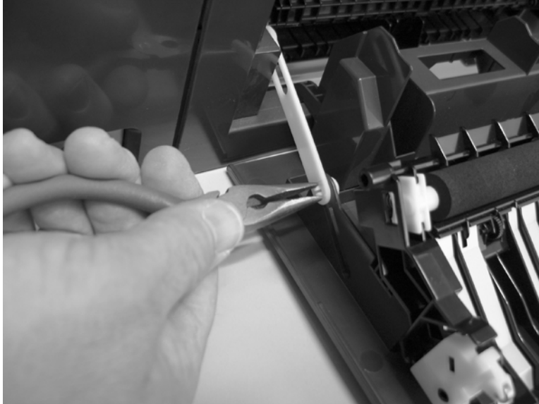
Figure 6-43 Remove the Rear-door stopper and link caps (simplex product) (1 of 2)
