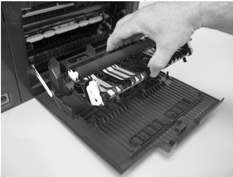
Figure 6-42 Remove the feed assembly (2 of 2)
