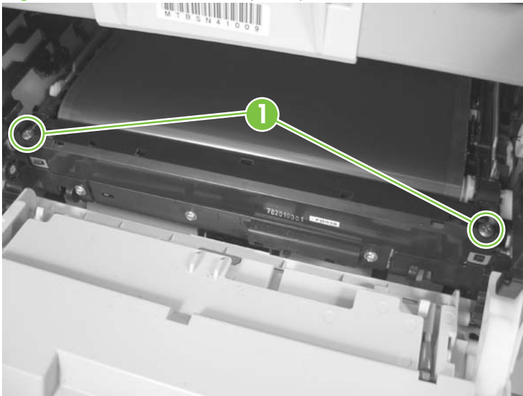
Figure 6-29 Remove the ITB (1 of 6)
