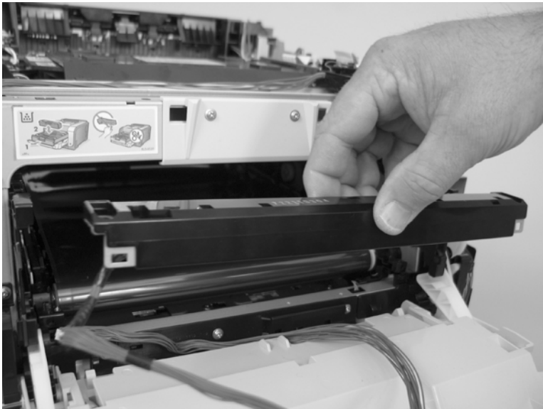
Figure 6-115 Remove the color-misregistration sensor assembly PCA (5 of 5)
