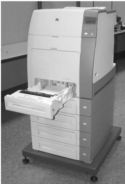
Figure 6-16 Remove the paper tray
