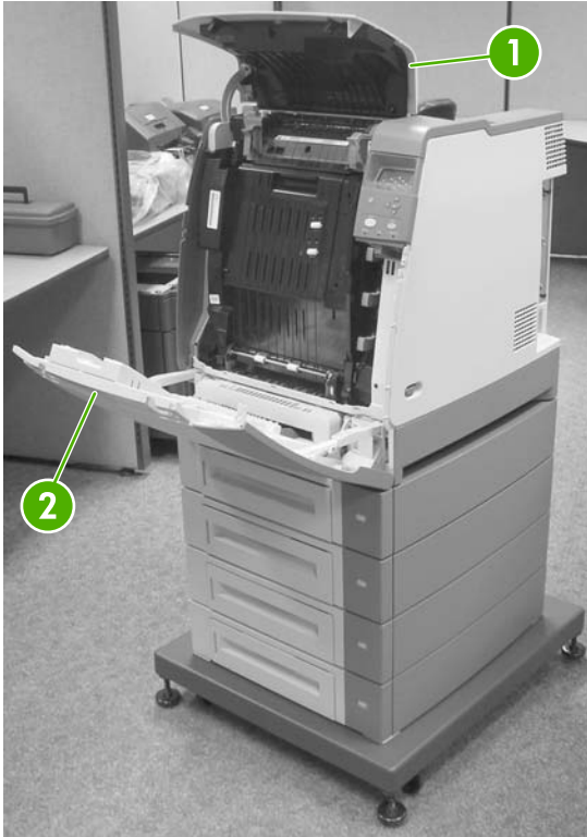
Figure 6-24 Remove the front cover (1 of 6)
