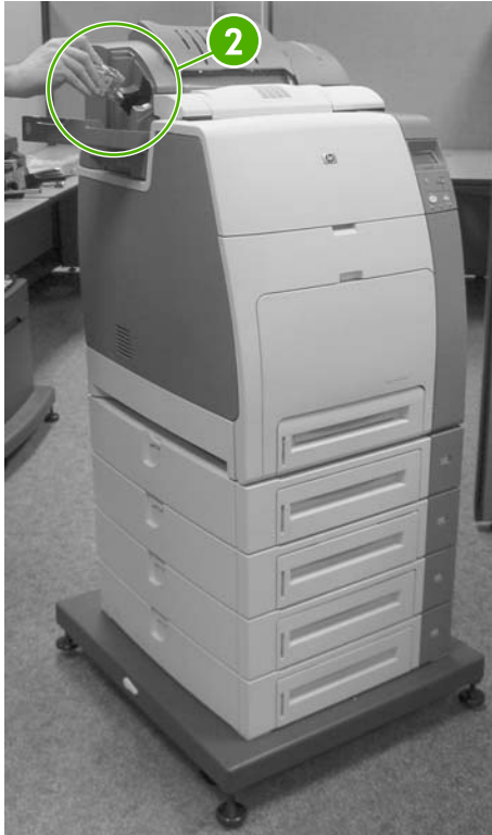
Figure 6-194 Remove the staple cartridge (2 of 2)
