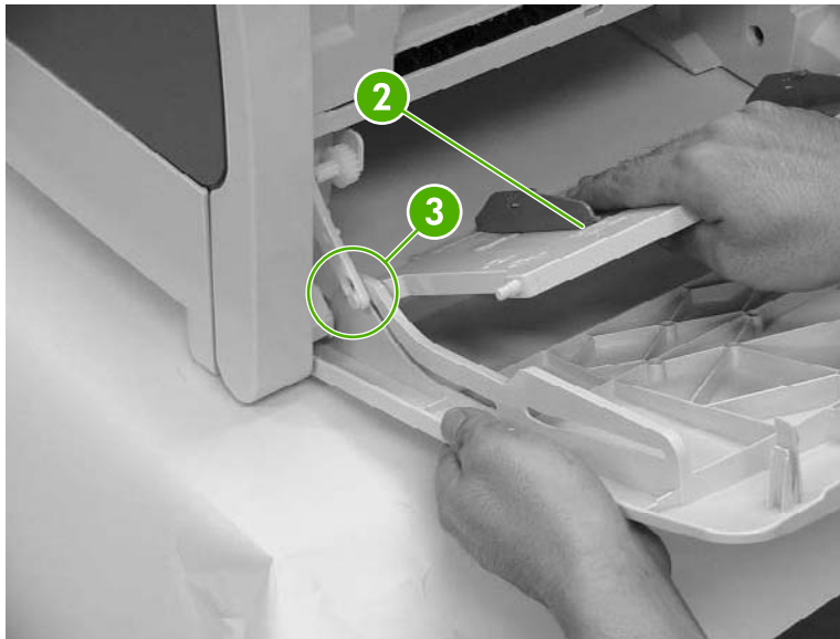
Figure 6-19 Remove the multipurpose tray (3 of 7)
