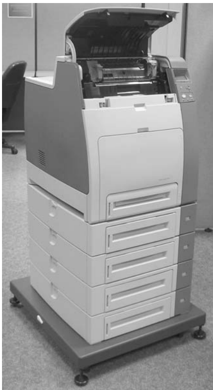
Figure 6-34 Remove the top cover (2 of 7)
