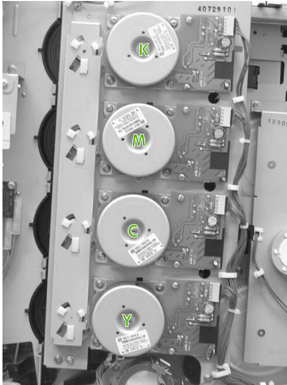
Figure 6-79 Reinstall the main drive assembly (16 of 16)
