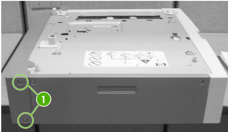
Figure 6-161 Remove the right cover (1 of 2)
