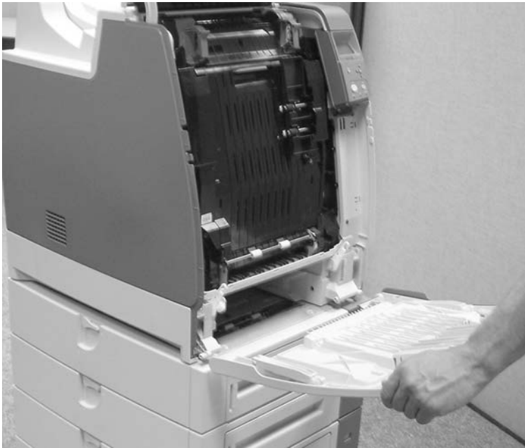
Figure 6-29 Remove the front cover (6 of 6)
