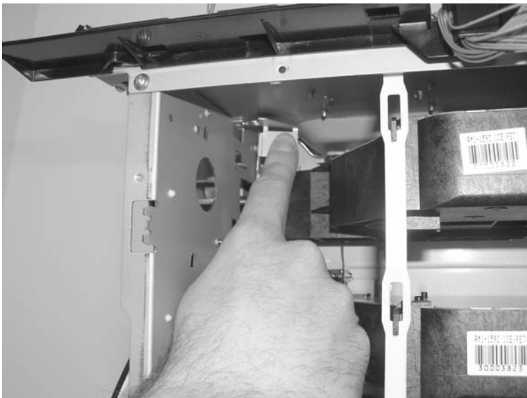
Figure 6-112 Remove the laser/scanner assembly (10 of 17)
