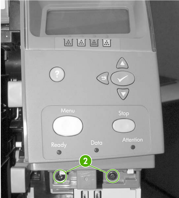
Figure 6-50 Remove the control panel (2 of 3)
