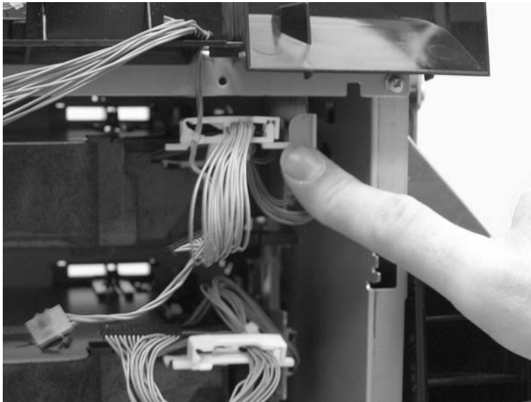
Figure 6-114 Remove the laser/scanner assembly (12 of 17)
