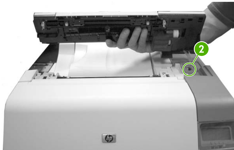
Figure 6-198 Remove the top duplexing assembly (2 of 2)
