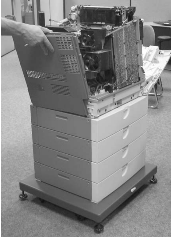
Figure 6-48 Remove the rear cover
