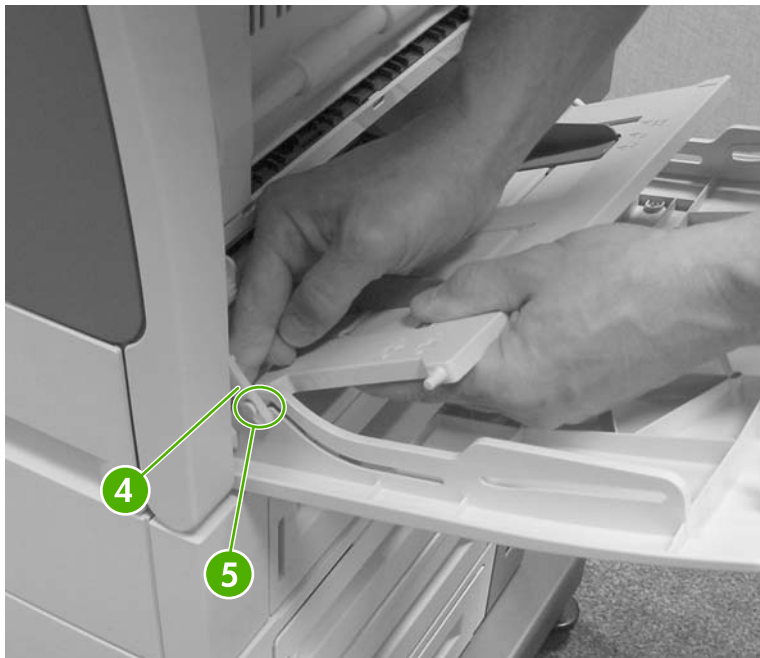
Figure 6-20 Remove the multipurpose tray (4 of 7)
