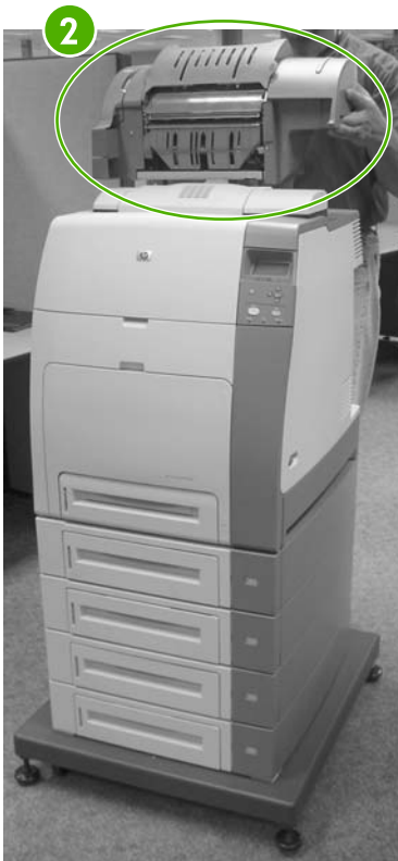
Figure 6-182 Remove the stapler/stacker from the printer (2 of 2)
