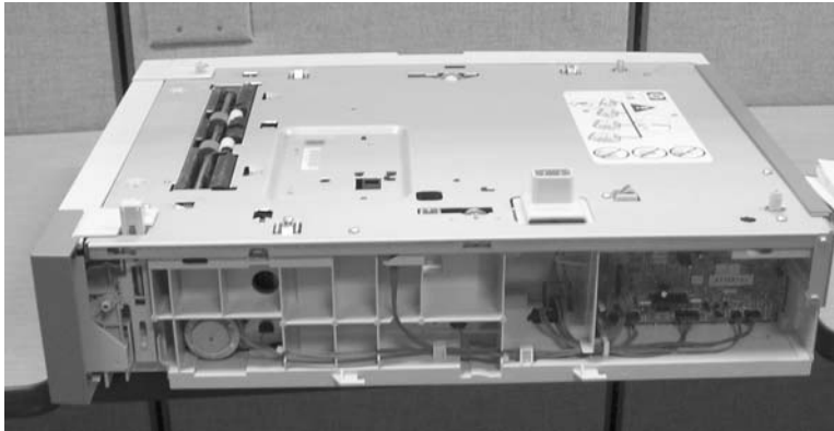
Figure 6-162 Remove the right cover (2 of 2)
