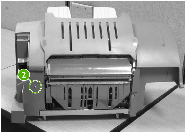
Figure 6-186 Remove the left cover (2 of 2)
