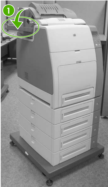
Figure 6-193 Remove the staple cartridge (1 of 2)
