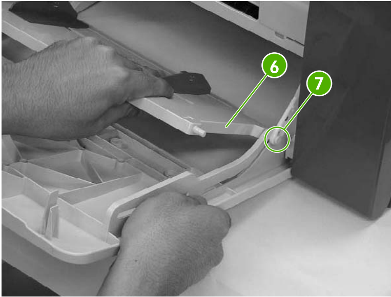
Figure 6-21 Remove the multipurpose tray (5 of 7)
