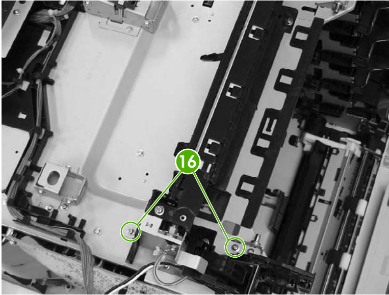
Figure 6-94 Remove the delivery assembly (8 of 9)
